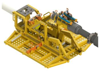
3. Flexible Riser and Pullhead assembly is lowered into place on to the porch structure.
