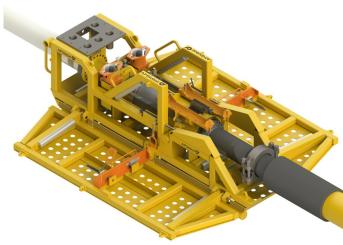
6. Annulus back seal pressure test performed, ROV tooling recovered, and the pipeline connection is complete.
