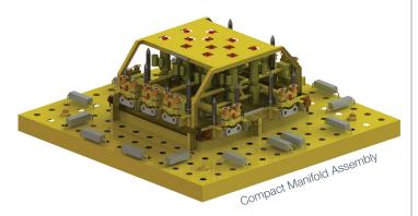
The AFGlobal compact manifold offers a direct weight savings of 25-40 percent with an equally discounted footprint. The piping kit of the compact manifold eliminates all 5D bends in the manifold structure (5D bends do not allow for a reduced structure height). This kit can reduce the piping weld count by 50 percent or more. This significant reduction in piping welds translates to a lower cost, shorter schedule, and reduced risk associated with subsea manifold fabrication.
