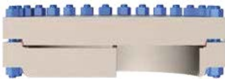
New Design with Taper-Lok Pressure Seal (No Diaphragm)
